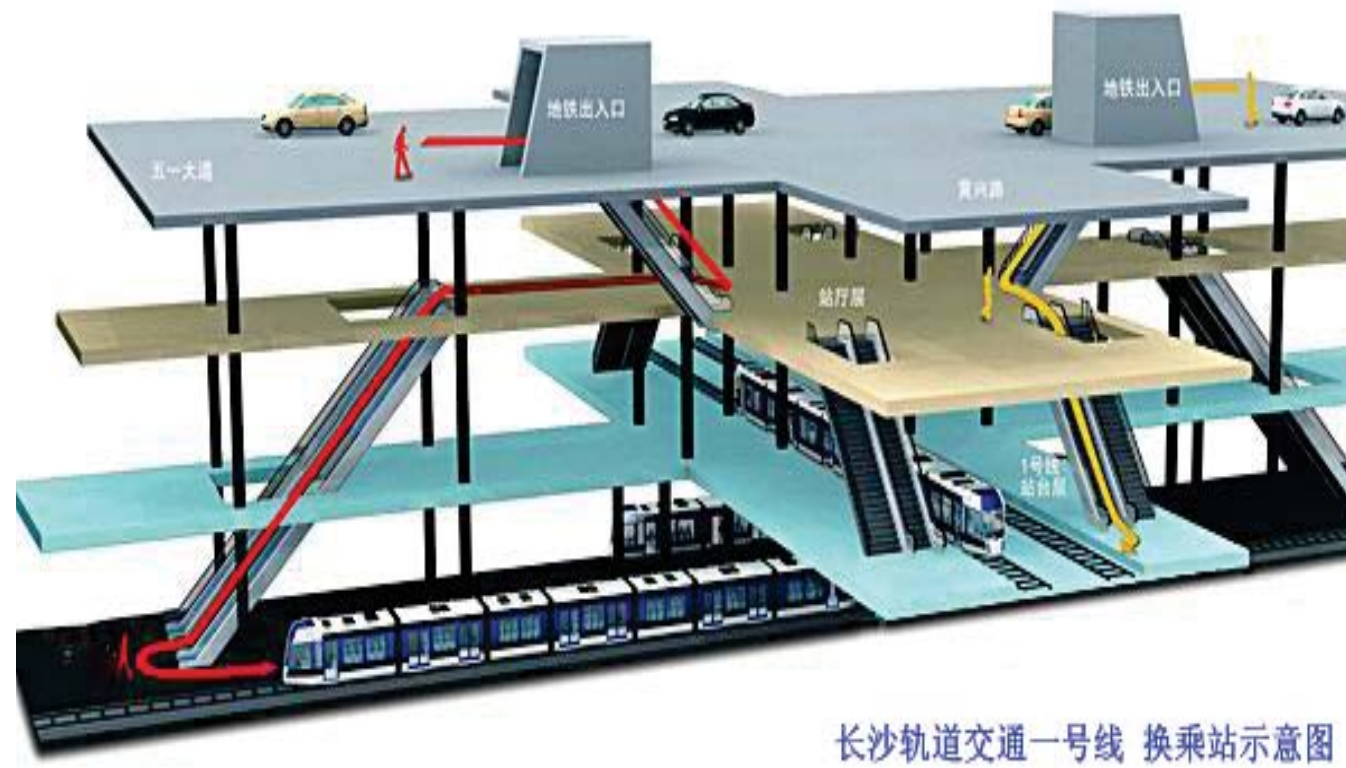
Changsha Metro Line 1 (103)
